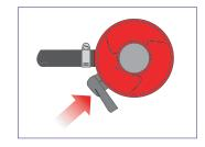
**4 Replacement of a cylinder** Ensure that all taps on the gas appliances are in the OFF position. The regulator lever is in the OFF position.
