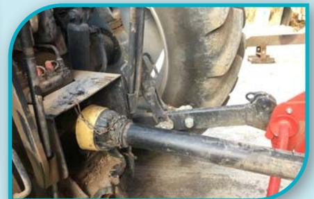
The P.T.O. takes the power from a tractor engine to run a piece of equipment such as a mower or agitator.
