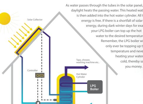
daylight heats the passing water. This heated water is then added into the hot water cylinder. All this energy is free. If there is a shortfall of solar energy, during dark winter days for example, your LPG boiler can top up the hot water to the desired temperature. Remember, the LPG boiler will only ever be topping up the temperature and never heating your water from cold, thereby saving you money.
