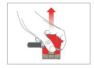
6 Pull upwards at the same time as pressing in the lever horizontally.
